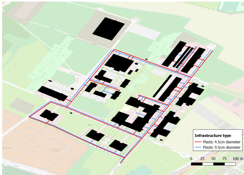
Figure 3.2: Spatial extent of the study area with data curated from OpenStreetMap and a utility network in the CityGML Utility Network ADE standard.
