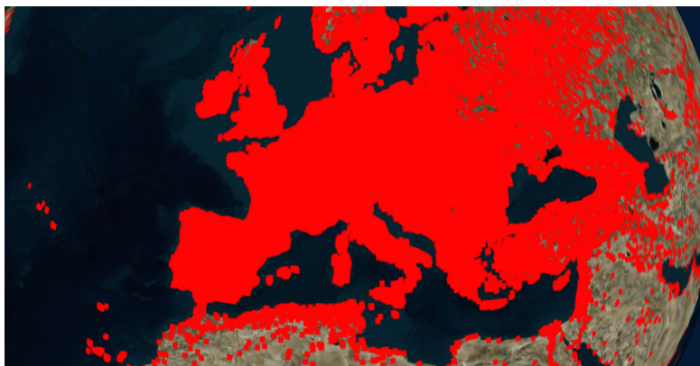
Figure 2.1: Glob3 Mobile web visualization of a dataset representing cities in the world. Displaying the raw dataset produces the undesirable cluttering effect.
