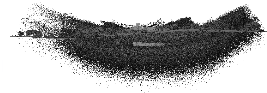
Figure 8.8: Point cloud heavily affected with arched and tubular noise artifacts. The density of noise points is high enough to make pointing out which points are representing terrain or trees hard, even with the human eye.
