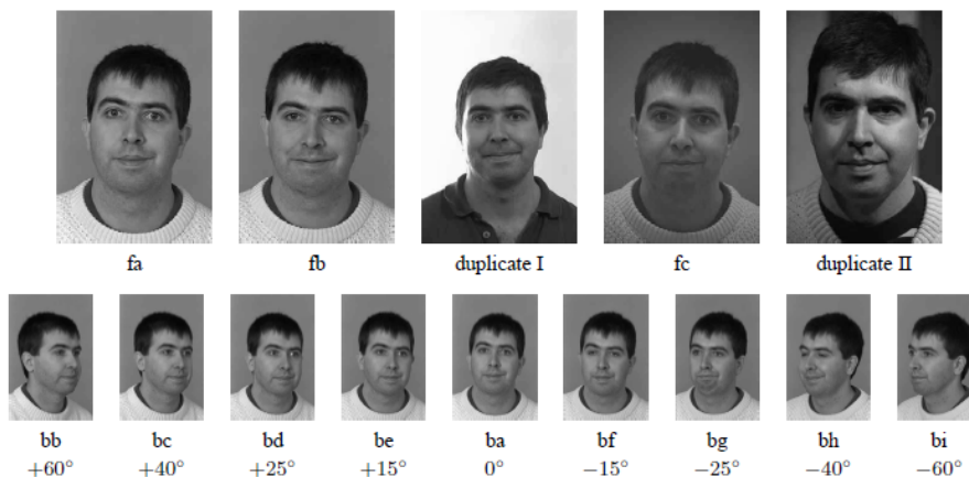
Figure 1.6: Frontal image and pose variation categories used in the FERET [42] evaluations. The duplicate I image was taken within one year of the fa image and the duplicate II and fa images were taken at least one year apart. Also, it can be appreciated that poses vary from +60. ( bb ) to full frontal ( ba ) and on to -60. ( bi ).
