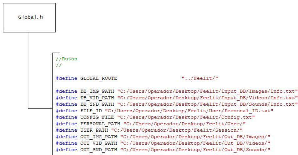
Figure 2.10: The Global.h file specifies all the paths used during the experiment. There are paths for the input data (DB_XXX_PATH) and for the output data (OUT_XXX_PATH). There are also detailed the PERSONAL_PATH (where is placed all private information about participants) and the USER_PATH (place where session information is saved). FILE_ID is an important file that keeps the relation between each participant PIN and its ID (See Fig. 2.13).
