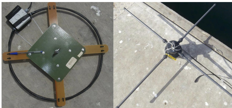
Figure 4. Antenna examples: on the left 22 cm magnetic loop and insulated crossed-dipole on the right.
